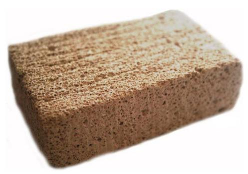
These lightweight properties mean that pumice is often used as a component in cinder blocks. Its rough surface also means that it is useful as an exfoliating (scrubbing) tool.
