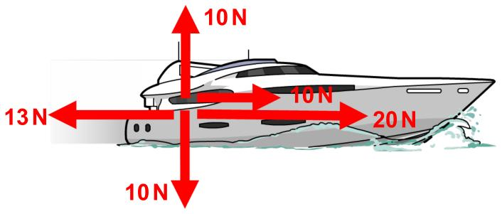
The vertical forces are equal in size and opposite in direction so there is no resultant force in the vertical direction.
