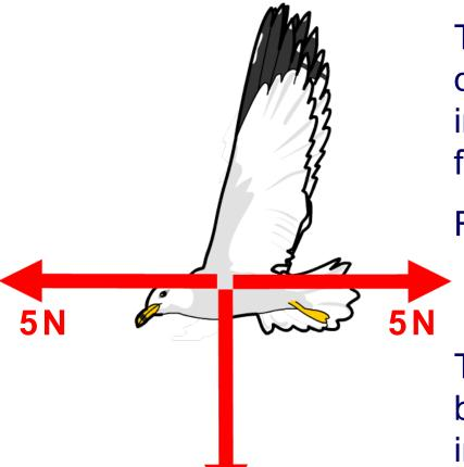
The forces acting in each direction horizontally are equal in size, so there is no resultant force in this direction.
