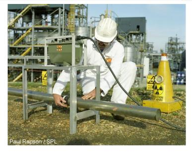
If a gamma source is placed on one side of the welded metal, and a photographic film on the other side, any flaws will show up on the film like an X-ray.
