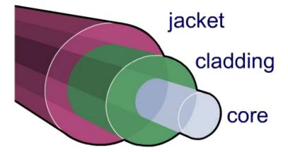
The glass core is often encased in a layer of cladding, which prevents light escaping the core. A protective plastic jacket surrounds the whole fiber.
