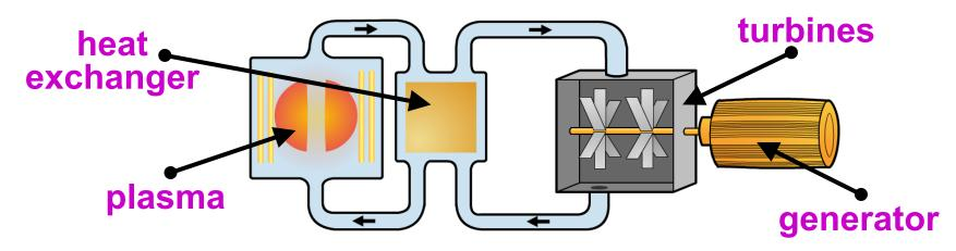
Then, like fossil fuel and fission power stations, the steam will drive turbines to produce electricity.
