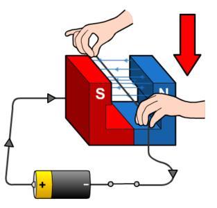
The direction of the force is, therefore, relative to both the direction of the magnetic field and the current.
