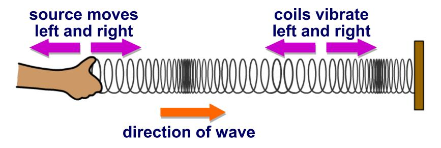
The wave travels away from the source. The direction of the wave is parallel to the movement of the source.
