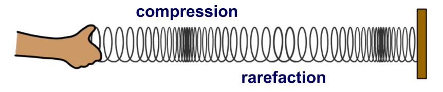
Sound waves are longitudinal waves. When someone speaks, the air particles vibrate as a longitudinal wave, and so compressions and rarefactions are formed in the air.
