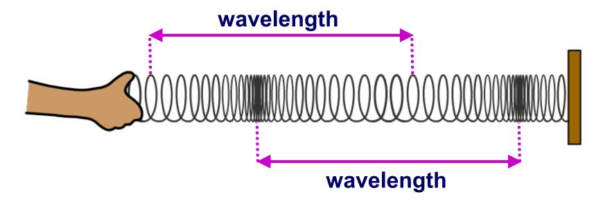
The wavelength is the same whichever two matching points are used to measure this distance.
