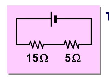
Total resistance =  $R_1 + R_2$ =  $15\Omega + 5\Omega$ =  $20\Omega$
