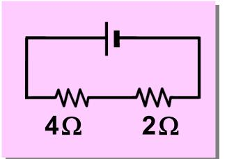
Total resistance =  $R_1 + R_2$ =  $4\Omega + 2\Omega$
