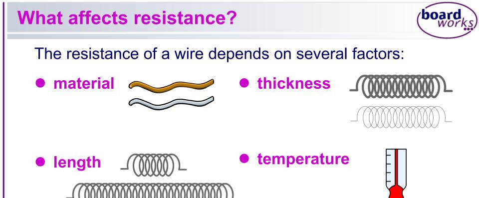
For example, a copper wire has a lower resistance than a nichrome wire of the same size. Copper's excellent ability to conduct electricity means it is often used in wiring.
