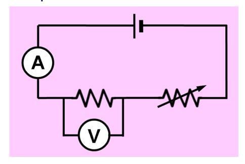
Slowly move the variable resistor so that the voltage increases by 0.5 V and record the current for each setting.
