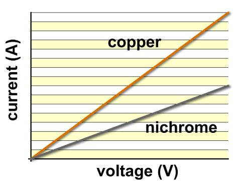
This means that the copper wire has a lower resistance than the nichrome wire. What does the gradient tell you about resistance?
