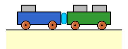
trolley B mass = 5 kg velocity = -4 m/s momentum = 5 × -4= -20 kg m/s
