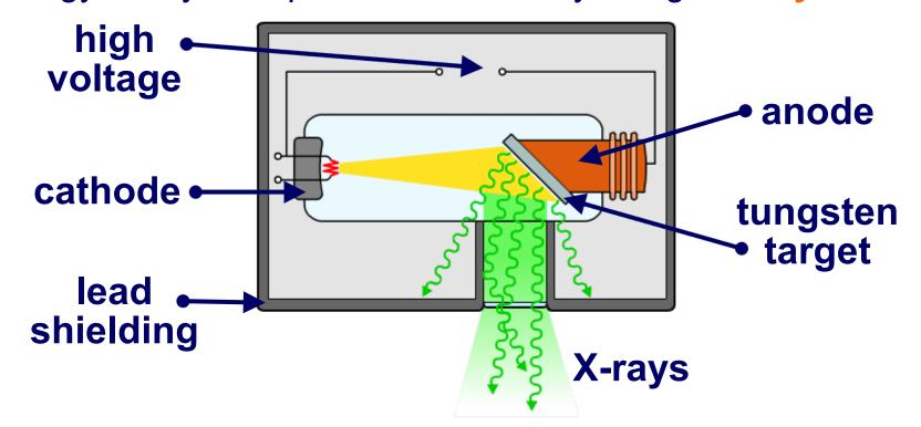
Electrons from the hot cathode are fired at the tungsten target at high speed. When these high-energy electrons strike the target, some of their energy is changed into X-rays.
