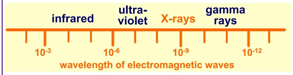
X-rays have a very short wavelengths between 0.1 and 10 nm. (The size of a water molecule is about 0.3 nm.)
