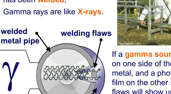
If a gamma source is placed on one side of the welded metal, and a photographic film on the other side, any flaws will show up on the film like an X-ray.
