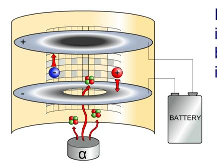
If there is smoke present, it interacts with the ions produced by the alpha particles and ionization is reduced.
