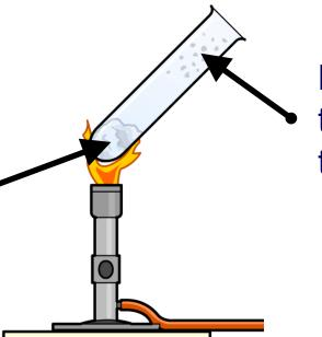
NH<sub>4</sub>Cl reforms in the cooler part of the test tube
