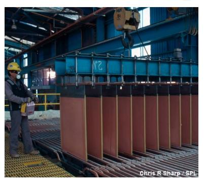
This process is carried out on a huge scale in industry, and the copper formed on the negative electrodes is 99.99% pure.
