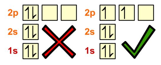
Hund's rule states that single electrons occupy all empty orbitals within a sublevel before they start to form pairs in orbitals.
