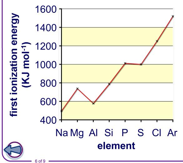
However, sulfur's value is below that of phosphorus. As the highest energy electrons of both are in the 3p sublevel this is evidence for Hund's rule.
