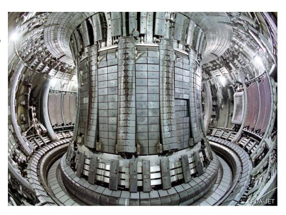
The reactor is most efficient as a doughnut shape.
