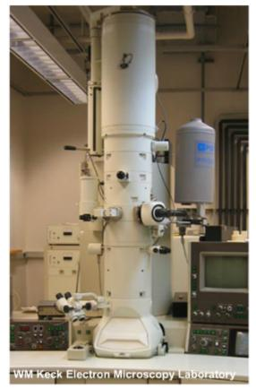
An **electron microscope** exposes a specimen to electrons instead of light. Electrons have a much shorter wavelength than light, which means they can produce images of much greater resolution (up to 0.1nm) and magnification (up to 2×10<sup>6</sup>) than those of a light microscope.
